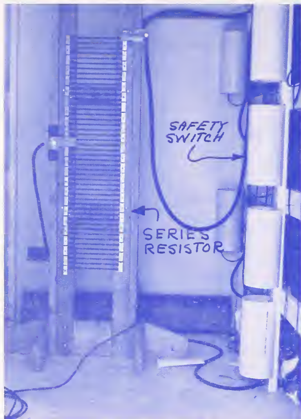
Figure 9—Part of the battery building interior. The series resistor carbon rod array is on the left. The movable tap is on the left side of the resistor array. The safety switches are covered for safety, and the use of the flag in the photograph of figure 8 is apparent.
